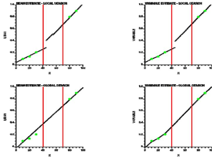
**Figure 6:** A simple 1D illustration of the importance of a global search in kriging with a trend (KT).
